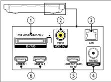
SD CARD-FOR VOD/BD-LIVE ONLY Slot for SD card. The SD card is used to rent online videos and access BD-Live.
