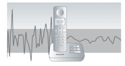
Automatic Volume Control offsets variations in sound signal, which can be caused by distance, signal strength or the caller's phone so what you hear always remains consistent. Reducing the audio amplification for strong signals, and increasing it for weak ones, it means you can enjoy a smooth conversation without unwanted sound volume variation.
