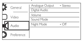
[Analogue Output] - Adjust this setting for audio output through AUDIO OUT L/R.
