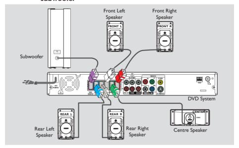
Connect the supplied speakers system using the fixed speaker cables by matching the colours of the sockets and speaker cables.
