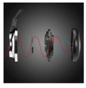
The Fidelio NC1 uses a feed-forward and feed-backward active noise cancellation (ANC) solution, which means there are 4 microphones implemented inside and outside the ear cans to capture noise for advanced processing. The feed-forward ANC (mic outside the ear can) covers a wider bandwidth of frequencies, while the feed-backward ANC
