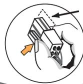
**3e** Connect the SonoWave Speakers to the AV subwoofer. (refer to next page for "Speaker system setting")
