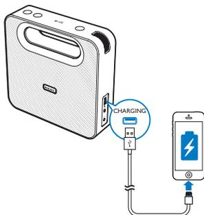
In AC power supply mode, connect to your mobile device with a USB cable (not supplied).
