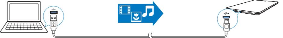
**EN** Use the USB cable to connect PI2010 to PC. You can drag and drop apps and media files between PI2010 and PC.
