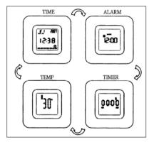
Rotate the clock clockwise in four directions to set the following functions:
