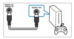
Using a coaxial cable, connect the COAXIAL connector on your SoundBar to the COAXIAL/DIGITAL OUT connector on the TV or other device. • The digital coaxial connector might be labeled **DIGITAL AUDIO OUT**.
