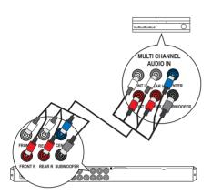
1 Connect the audio cables (not supplied) to the AUDIO OUT (FRONT L/R, REAR L/R, CENTER and SUBWOOFER) sockets on this DVD player and the audio input sockets on the device.
