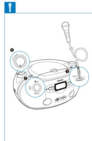
When use a low sensitivity microphone, press MIC VOL up to HI to increase microphone loudness.
