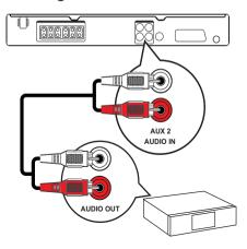
Connect the audio cables (not supplied) to the AUDIO IN-AUX2 sockets on the Home Theatre System and the AUDIO output sockets on the device.
