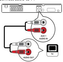
1 Connect the audio cables (not supplied) to the AUDIO IN-AUX1 sockets on the Home Theatre System and the AUDIO output sockets on the TV.
