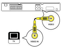
1 Connect a composite video cable to the VIDEO socket on this Home Theatre System and the VIDEO input socket on the TV.
