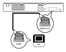
1 Connect a scart cable (not supplied) to the SCART TO TV socket on this Home Theatre System and the SCART input socket on the TV
