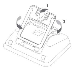
**3** Re-insert the bracket into the back of the base station.
