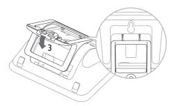
4 Insert screws (not included) into the wall.
