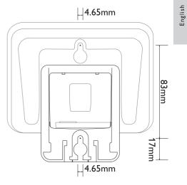
5 Align the mounting holes on the back of the base station with the screws on the wall.
