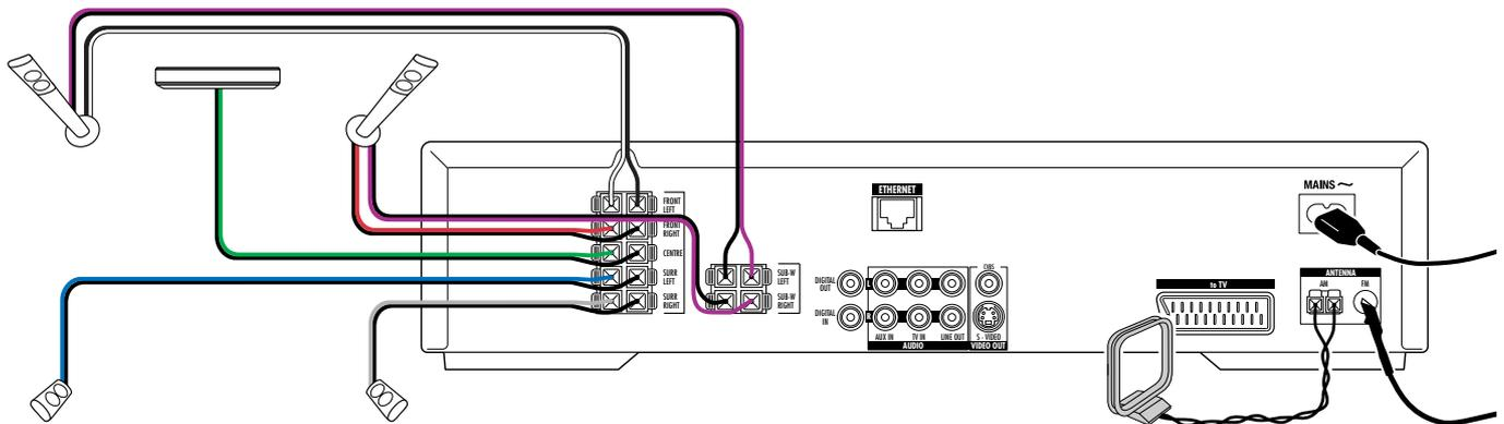
**5** Connect the speaker cables to the Streamium System.
