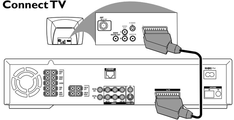
Connect the Scart socket on the TV to the Scart socket (to TV) on the Streamium System with the supplied Scart cable. If your TV has no Scart socket, please see page 12 of the user's manual.
