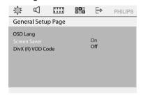
If Screen Saver set to On, the screen saver will be activated when you leave the system in stop or pause mode for 5 minutes. The default setting is "On".
