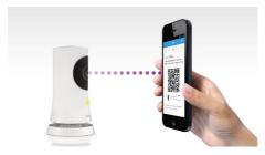
Set-up is simple with the In.Sight+ app. The app will generate a QR code for your home Wi-Fi settings. With the QR code, the monitor will automatically pair with your Wi-Fi network, easily and instantly.
