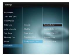
→ If you select [RadiantColor], the PhotoFrame extends the color on the edges of a photo that is smaller than the full screen to fill the screen without black bars or aspect ratio distortion.
