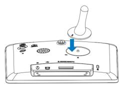
2 Turn the stand anti-clockwise 45 degrees to the å position and lock it to the PhotoFrame firmly.
