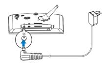
2 Connect the power cord to a power supply socket.
