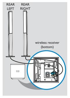
Step 3: Connecting the rear speakers to wireless receiver
