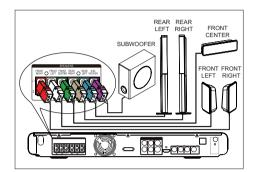
1 Connect the speakers and subwoofer to the matching sockets on this unit.
