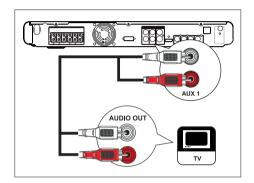
Connect an audio cable (not supplied) from the AUDIO IN-AUX1 sockets on this unit to the AUDIO OUT sockets on your TV.
