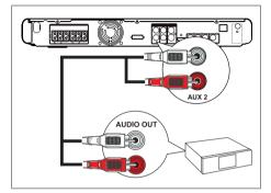
Connect an audio cable (not supplied) from the AUDIO IN-AUX2 sockets on this unit to the AUDIO OUT sockets on the device.
