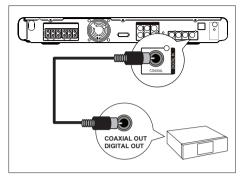
1 Connect a coaxial cable (not supplied) from the **DIGITAL IN-COAXIAL** socket on this unit to the COAXIAL/DIGITAL OUT socket on the device.
