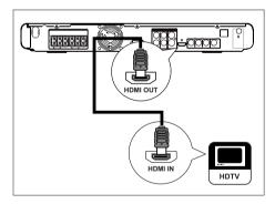
1 Connect a HDMI cable (not supplied) from the HDMI OUT on this unit to the HDMI IN socket on your TV.
