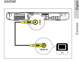
1 Connect a composite video cable (yellow supplied) from the VIDEO OUT-CVBS socket on this unit to the video input socket on your TV.
