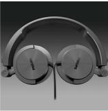
the DJ monitoring style headphones can be easily folded away for perfect portability and storage. Its clever design features careful selection of components, like well-built hinges, that allow the headphone parts to be maneuvered with ease. The SHL3050 can be folded flat or inwards, for a compact fit on the go.
