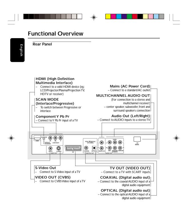
Caution: Do not touch the inner pins of the jacks on the rear panel. Electrostatic discharge may cause permanent damage to the unit.
