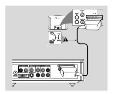
Use the SCART cable (black) to connect the DVD Player's SCART jack to the corresponding Scart input jacks on the TV (cable not supplied).
