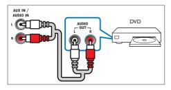
Using an analog cable, connect the AUX connectors on your SoundBar to the AUDIO OUT connectors on the TV or other device.
