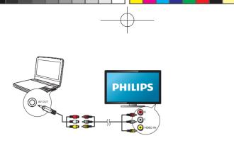
Match the color of the AV cables (the AV cable connected to TV is not supplied) with the jacks:
