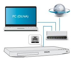
• For Wi-Fi, connect a Philips Wi-Fi USB adapter (named WUB1110) to the • ← (USB) connector on the front panel of this player.
