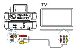
As shown, plug the supplied composite audio/video cable into the corresponding sockets.
