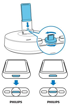
Slide the connector to the center of the device.
