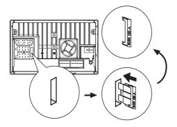
If the fuse gets damaged immediately after it has been replaced, there may be an internal malfunction. In such case, consult your Philips dealer.
