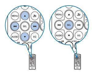
3 Press I ← or ►►I to tune to a radio station manually.
