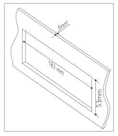
5 Install the sleeve into the dashboard and bend the tabs outward to fix the sleeve.
