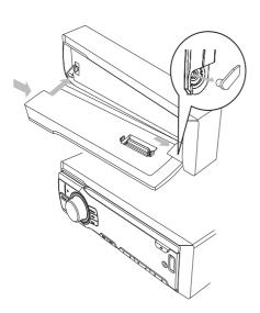
Insert the right side of the panel in the chassis until it is correctly engaged.
