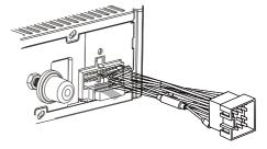
3 Connect the antenna and amplifier as illustrated, if applicable. You can connect the car audio to the amplifier through RCA-TO-RCA cables (not supplied).
