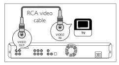
1 Connect a RCA video cable (supplied) to the VIDEO OUT socket on this unit and the video input socket on your TV.
