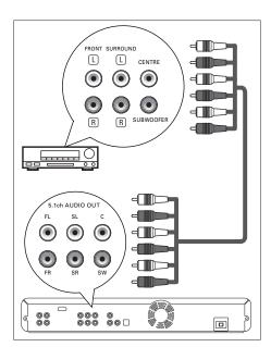
1 Connect a 5.1ch audio cables (not supplied) to the **5.1ch AUDIO OUT** sockets on this unit and the audio input sockets on the device.
