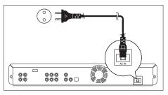
After you made all the necessary connections, connect the AC cord to the AC IN on this unit and to the AC power outlet.
