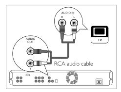
1 Connect an RCA audio cable (supplied) to the AUDIO OUT sockets on this unit and the AUDIO IN sockets on your TV.
