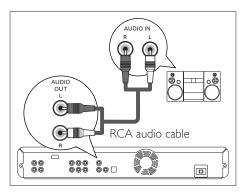
1 Connect an RCA audio cable (supplied) to the AUDIO OUT sockets on this unit and the audio input sockets on the device.
