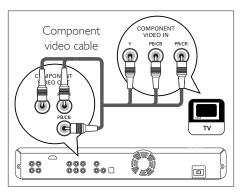
1 Connect the component video cable (not supplied) to the COMPONENT VIDEO OUT socket on this unit and the component video input sockets on your TV.
