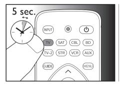
Point at your device with the universal remote. Then press and release U to start searching the code for your brand. A different infrared signal is sent every 2 seconds as the universal remote searches, indicated by a red flash.
