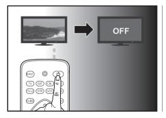
4 When the device is off, immediately press and release OK to save the code. The red LED indicator will turn off.
