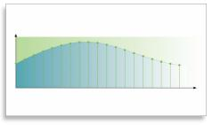
192KHz sampling enables you to have an accurate representation of the original sound curves. Together with a 24-bit resolution, more information is captured from the original analogue sound wave form, giving a much richer audio reproduction.
