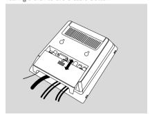
Align the side marked PRESS▼ of the stand to the slots at the bottom of the set.
