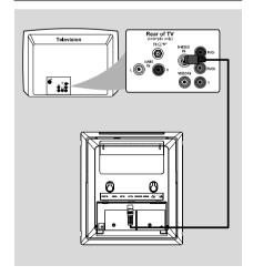
Use the S-Video cable (not supplied) to connect the system's S-VIDEO jack to the S-Video input jack (or labeled as Y/C or S-VHS) on the TV set.
