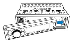
Press the left end of the front panel inwards until it is securely locked with a "click".
