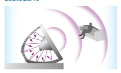
The carefully designed curved back cover of this Philips docking speaker creates a highly effective acoustic structure for sound reproduction. Its clean curve enforces the rigidity of the speaker cabinet, dramatically reducing internal resonance and eliminating the vibration and distortion of sound. You get to enjoy superb crystal-clear sound in stunning looking speakers.
