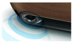
Bass-reflex acoustic load uses a bass pipe tuned to the acoustic volume of the speaker box, in order to reproduce deep bass from compact enclosures. The carefully designed profiled bass-pipe helps air flow and allows for deep and impactful bass, even at loud volumes while minimizing air turbulence that may cause distortion.
