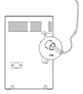
Connect the FM antenna to the FM ANTENNA socket on the back panel.
