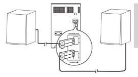
Connect the speaker cable plugs to the **SPEAKER OUT** sockets.
