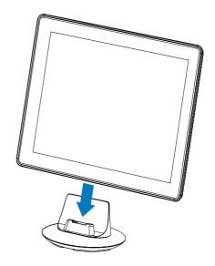
→ If the PhotoAlbum is powered off, the LED indicators under the left-right slider and the **OK** button blink during the charging process. When the built-in battery is fully charged, the LED indicators stop blinking.
