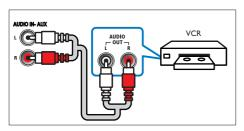
1 Using an analog cable, connect the AUX connectors on your home theater to the AUDIO OUT connectors on the TV or other device
