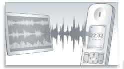
We test the sound quality of our DECT phones the same way as high-end headphone manufacturers do. Using an advanced ear simulator, we can accurately re-create the way people actually hear. This helps our acoustic engineers to measure and fine-tune things like frequency response, distortion and overall hearing perception, to create perfect voice reproduction for both handset and handsfree modes.
