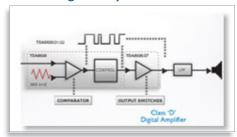
Class 'D' Digital Amplifier takes an analog signal, converts it into a digital signal and then amplifies the signal digitally. The signal then enters a demodulation filter to give the final output. The amplified digital output delivers all the advantages of digital audio, including improved sound quality. In addition, Class 'D' Digital Amplifier has greater than 90% efficiency compared to traditional AB amplifiers. This high efficiency translates into a powerful amplifier with a small footprint.
