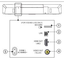
(1) SD CARD FOR VOD/BD-LIVE ONLY Slot for SD card. The SD card is used to access BD-Live only.
