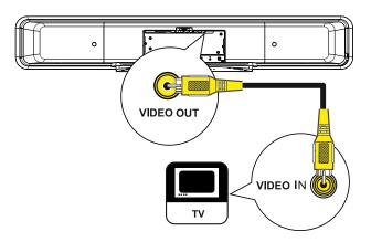
1 Connect a composite video cable (supplied) from the VIDEO OUT socket on this unit to the video input socket on your TV.
