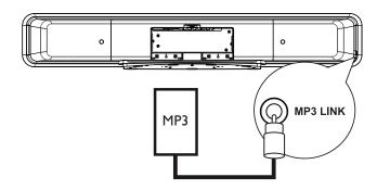
1 Connect a 3.5mm stereo audio cable (supplied) from the MP3 LINK socket on this unit to the phone socket on your portable media player (such as MP3 player).
