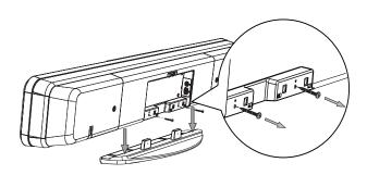
Attach the supplied knobs to the rear of this unit.
