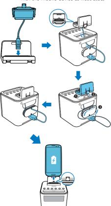
For Apple devices with a lightning or 30-pin connector: use the charging cable of the Apple device (not supplied) to connect the product with the mobile device as illustrated;
