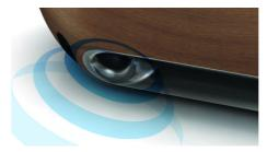
Bass-reflex acoustic load uses a bass pipe tuned to the acoustic volume of the speaker box, in order to reproduce deep bass from compact enclosures. The carefully designed profiled bass-pipe helps air flow and allows for deep and impactful bass, even at loud volumes while minimising air turbulence that may cause distortion.
