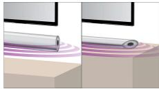
The quality of your sound experience is determined by how the soundbar is positioned in a room. Luckily, this system comes with a smart auto-orientation sensor that instantly optimizes audio quality once it detects whether your soundbar is placed horizontally or vertically. So, whether you choose to sit your soundbar on a shelf or mount it on a wall, you can be sure you'll always have a superb audio experience.
