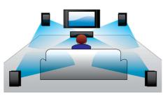
A built-in Dolby Digital decoder eliminates the need for an external decoder by processing all six channels of audio information to provide a surround sound experience and an astoundingly natural sense of ambience and dynamic realism. Dolby Pro Logic II provides five channels of surround processing from any stereo source.
