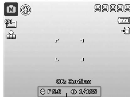
Displays the aperture and shutter speed value
