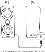
${\bf 2}$   $\,$  Connect the audio input plug to the audio output of your computer.
