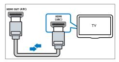
1 Using a High Speed HDMI cable, connect the HDMI OUT (ARC) connector on your SoundBar to the HDMI ARC connector on the TV
